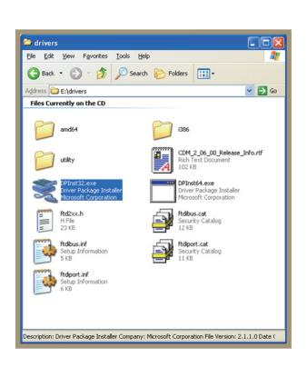
Insert the DVD and load the USB COM driver by executing the program \drivers\DPInst32.exe. For 64-bit systems execute the
