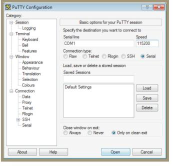
Open your preferred serial console window (TeraTerm, HyperTerminal, PuTTY) and connect to the COM port for the EVM using the these configuration settings.
