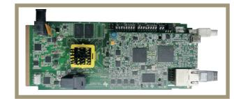
Connect the USB mini-B cable to USB1, Ethernet cable to Ethernet port (LAN1) and +12V DC power adapter to power jack(DC\_IN1). Ensure EVM configuration switches (SW3, SW5, and SW9) are set as shown.
