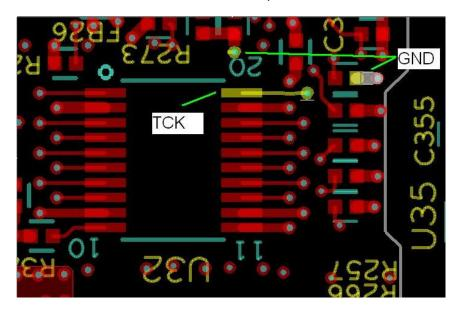
Figure 2. Location of TCK (U32.20) net and nearest GND nodes -- Bottom side of PCB
