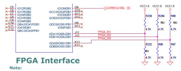
Figure 1: Board version resistor assembly
