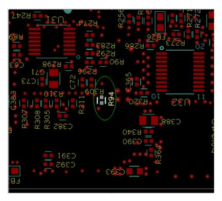
Figure 1. Location of R94 -- Bottom side of PCB near U32
