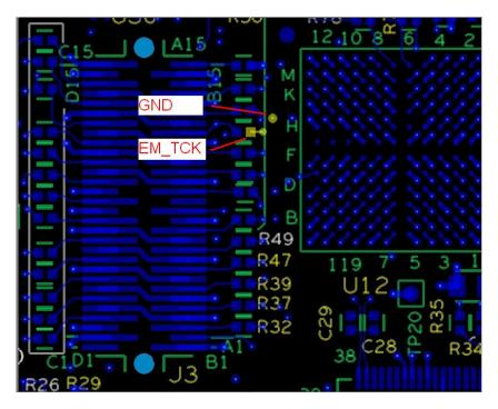
Figure 3. EM\_TCK net and nearest GND node -- Top side of PCB near 60 pin connector J3
