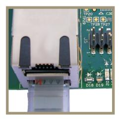
Connect Ethernet switch / router / PC to the lower Gigabit Ethernet port (J3) of TMDSEVM6472LE board using an Ethernet cable to access EMACO.
