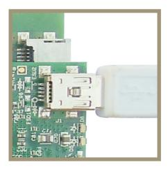
Connect the Mini-USB cable to J1 plug on XDS560v2 Emulator for high speed Emulation, as shown in figure. (For use with CCS debugger only)
