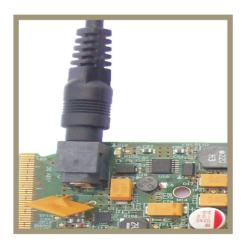
Connect the 12V DC power adapter (supplied with the kit) to power jack (J10).
