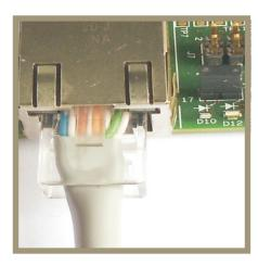
Connect Ethernet switch / router / PC to the Gigabit Ethernet port (J4) of TMDSEVM6457LE board using an Ethernet cable to access the EMAC port.
