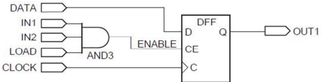
**Figure 2: Clock Enable - efficient way of gating a clock signal**
