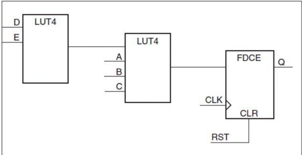
**Figure 3: Asynchronous reset implementation**
