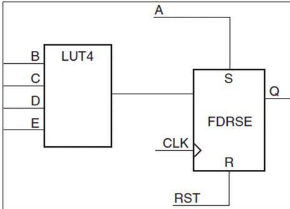
**Figure 4: Synchronous reset implementation**
