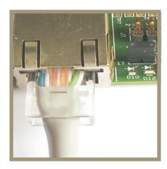
Connect Ethernet switch / router / PC to the Gigabit Ethernet port (J4) of TMDSEVM6457L board using an Ethernet cable to access the EMAC port.
