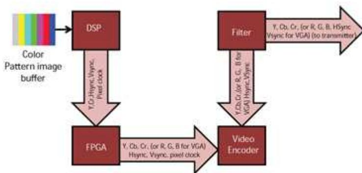
Figure 3: Here is an internal block diagram of the receiver.
