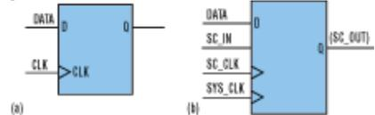
**2. Another scan approach replaces a design's ordinary flip-flop (a) with a clocked-scan cell (b).**
