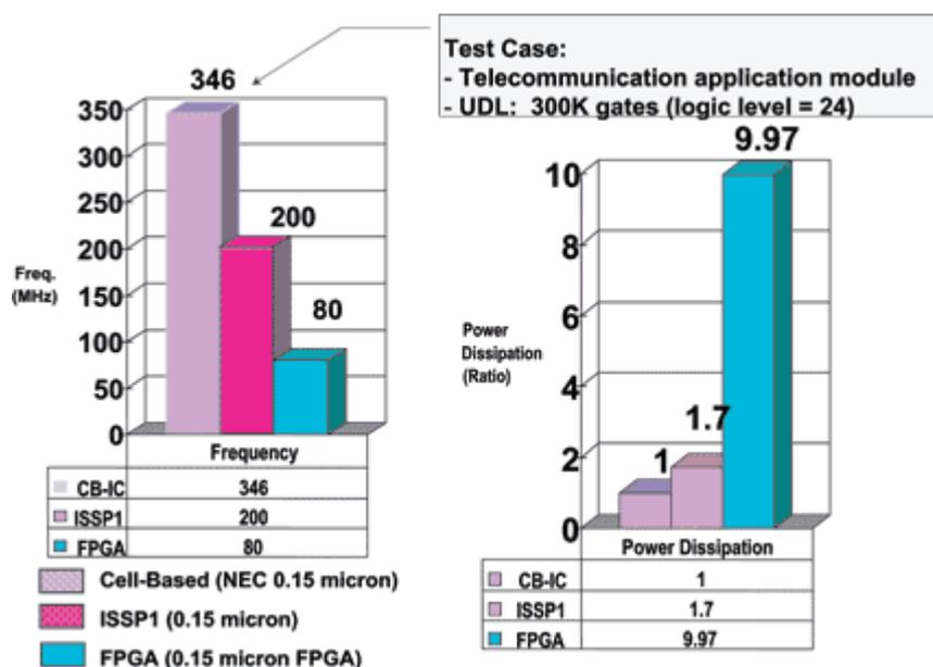
**Figure 1: This telecommunications-application study of a 150-nm, 300K-gate design shows the power consumption between FPGAs, structured ASICs, and ASICs.**
